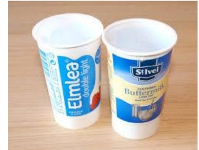
A thermoplastic sheet is clamped, heated, blown and stretched. Air is sucked out of the machine, forcing the softened sheet around a mould pushed up from below.
